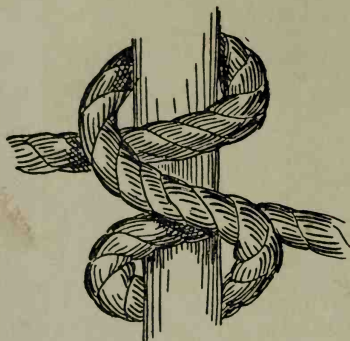
FIG. 36 A.—Clove hitch or builder's hitch (tying).
